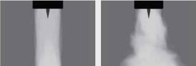
*The picture on the right shows a highly turbulent flow, offering poor shielding and elevated gas consumption.*
