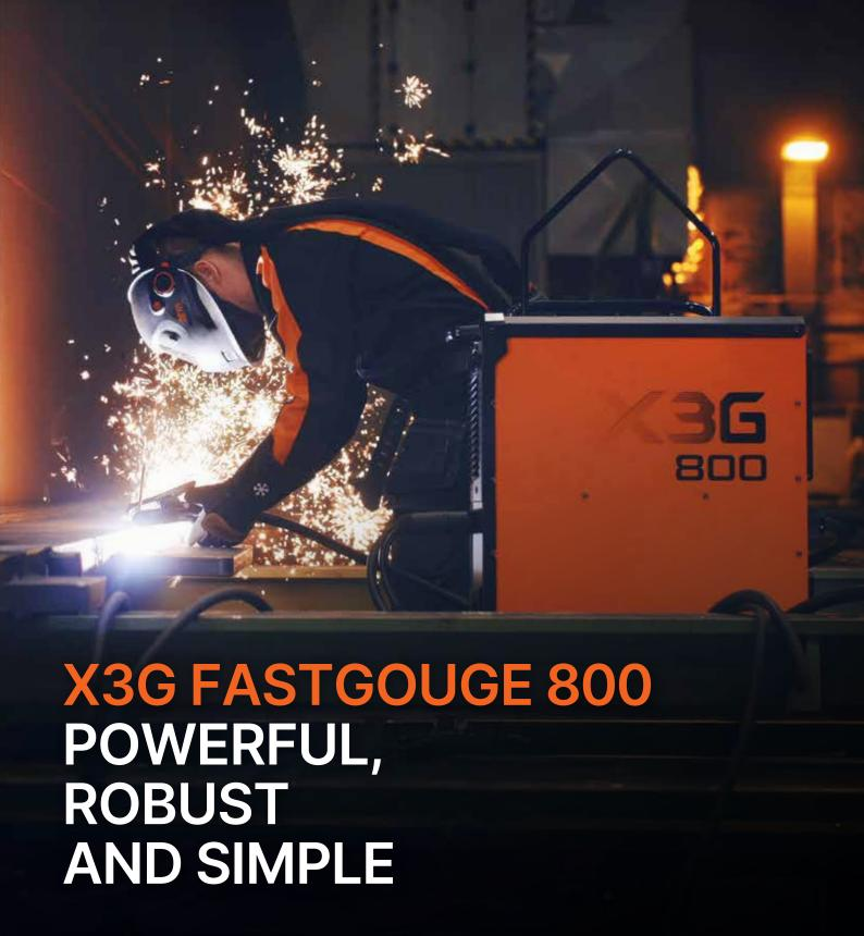
X3G offers a powerful, robust and simple solution for heavy-duty carbon arc gouging applications. 800 amps of power and a 50% duty cycle ensure maximum productivity and efficiency for those tough and challenging jobs.
