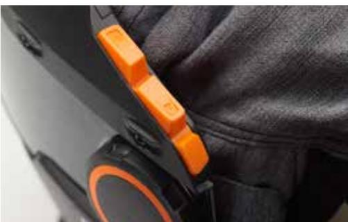
**Inboard mounted ADF remote control for reliability and convenience.** Remote control adjustment of the SA 60 or XA 74 automatic welding lenses features three silicon rubber selector switches. The large switches select parameter values up or down and the small switch selects either the parameter type, or a long press activates the work lights on the XFA model.
