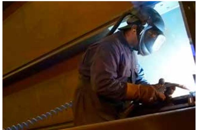
Supplied air solutions are ideal where welding gases may build up displacing breathing air.
